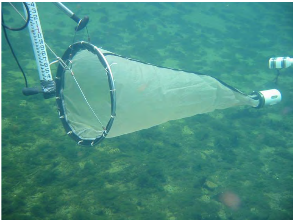
Figure 9. Image of plankton net capturing suspended material with flow meter upstream
