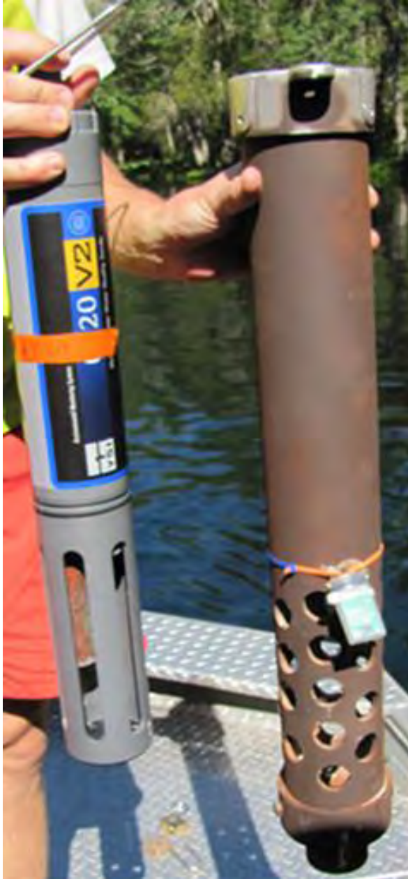
Figure 5. Image of data sonde housing with holes that allow free movement of water, while the locking cap and cable provide security.
