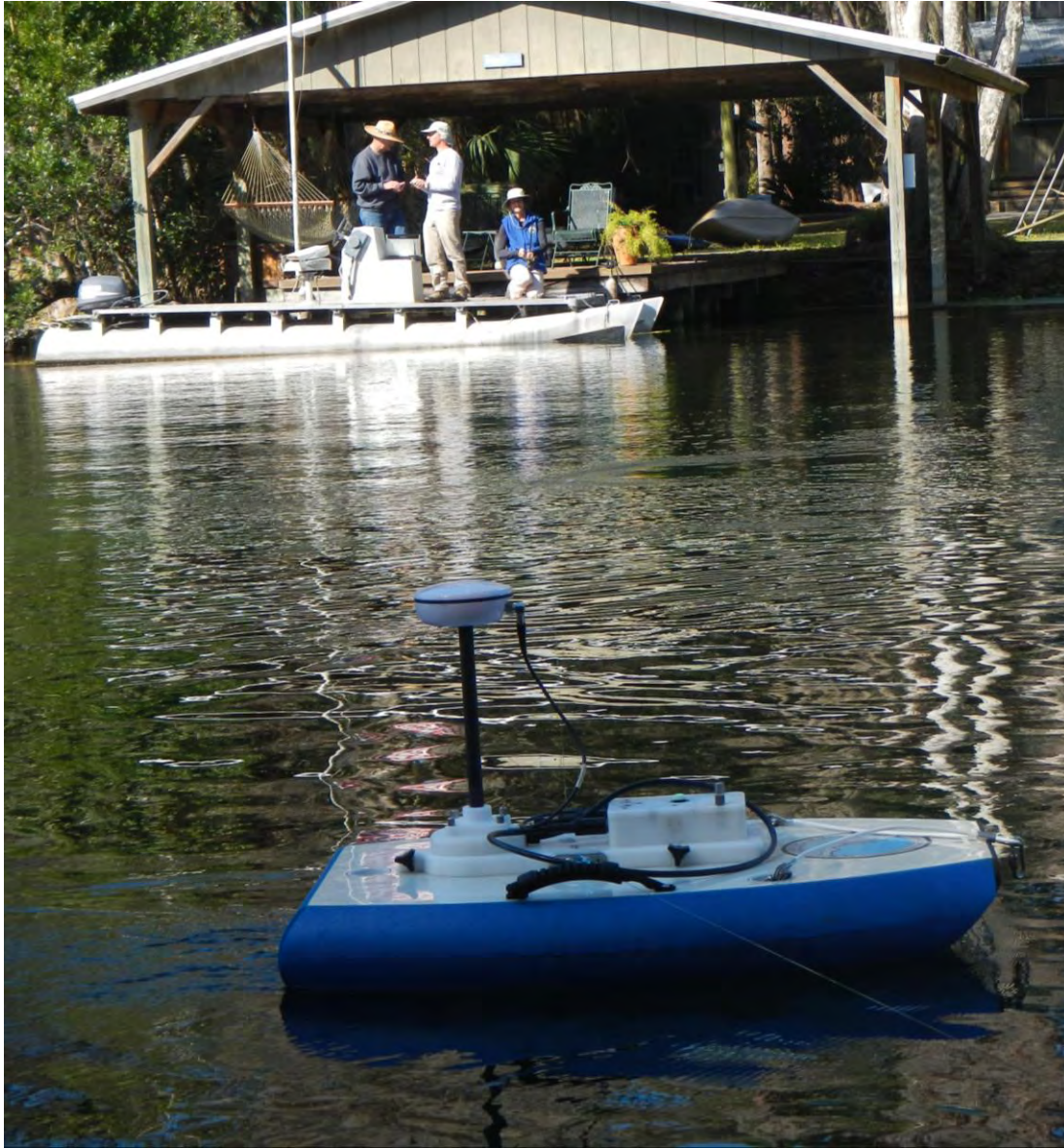
Figure 4. Stream discharge measurement collected along a cross-section of the Rainbow River.
