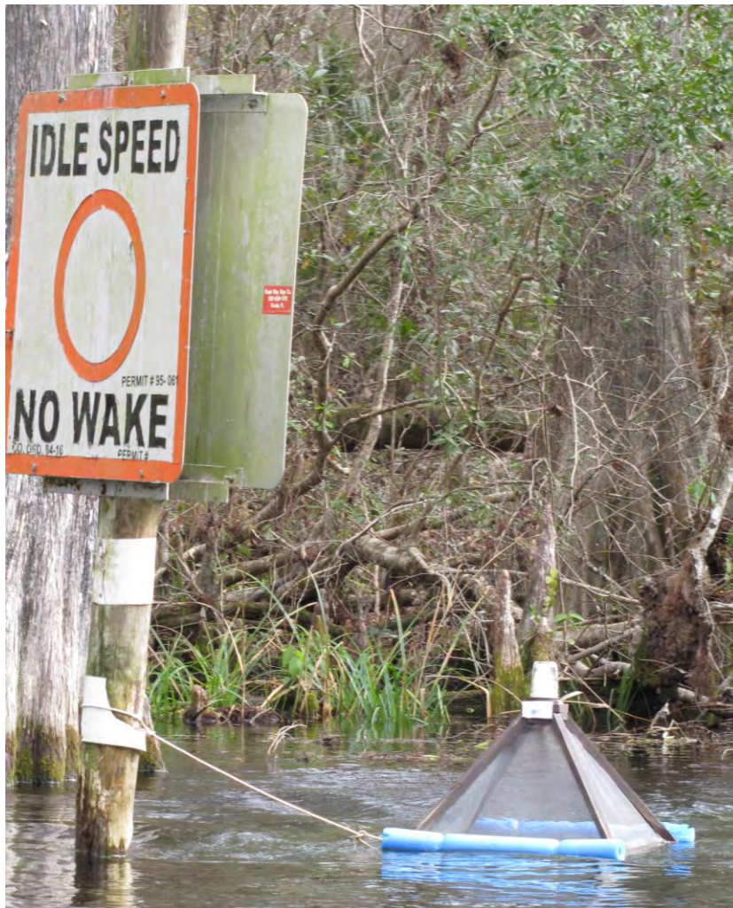
Figure 6. Trap used to collect adult aquatic insects as they emerge from the water
