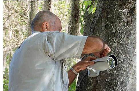
Installation of river monitoring video camera
